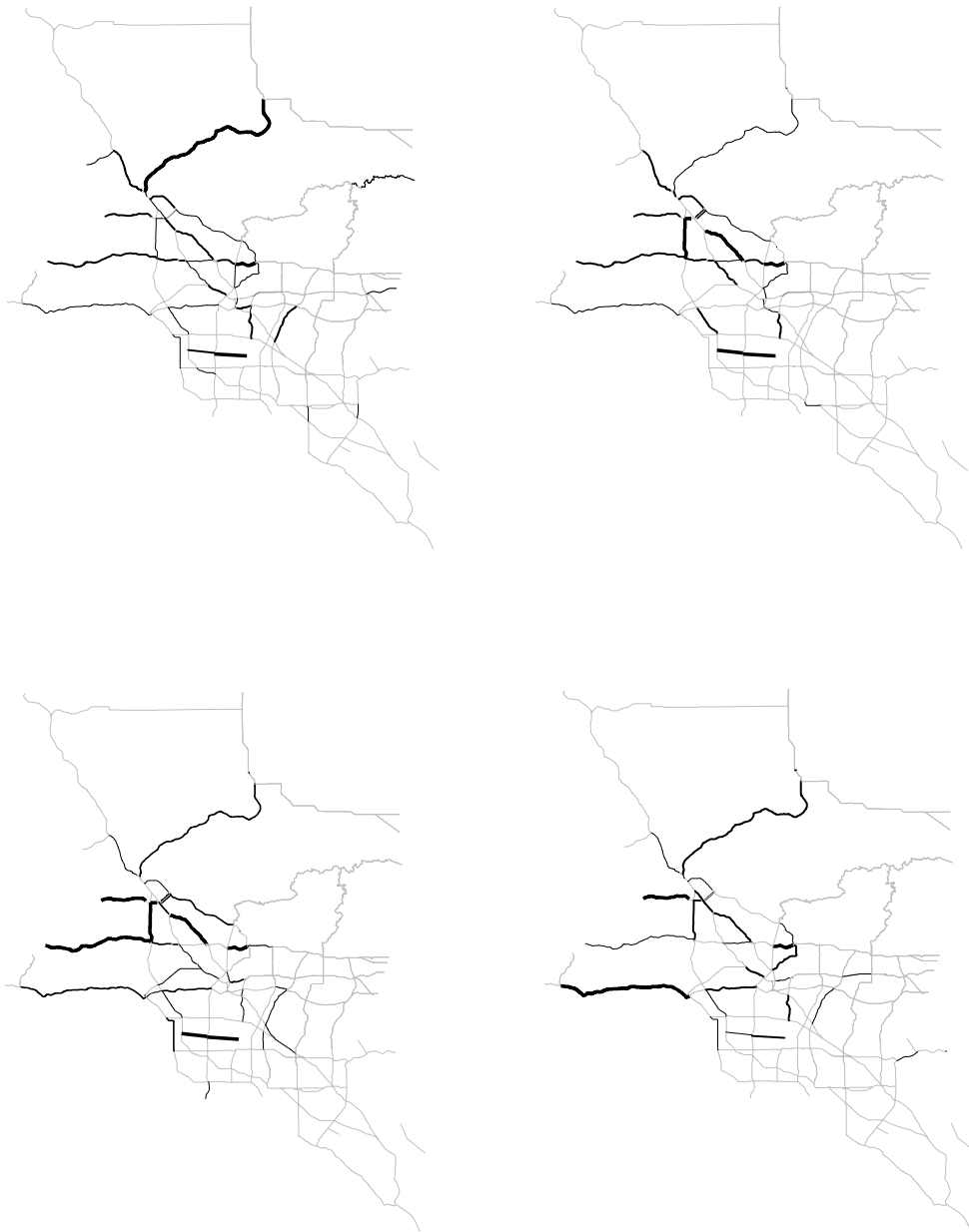
Figure A2-4: Simulated Bridge Failures Given Conditions Consistent with the Northridge Earthquake: Darker Links Have More Failures
