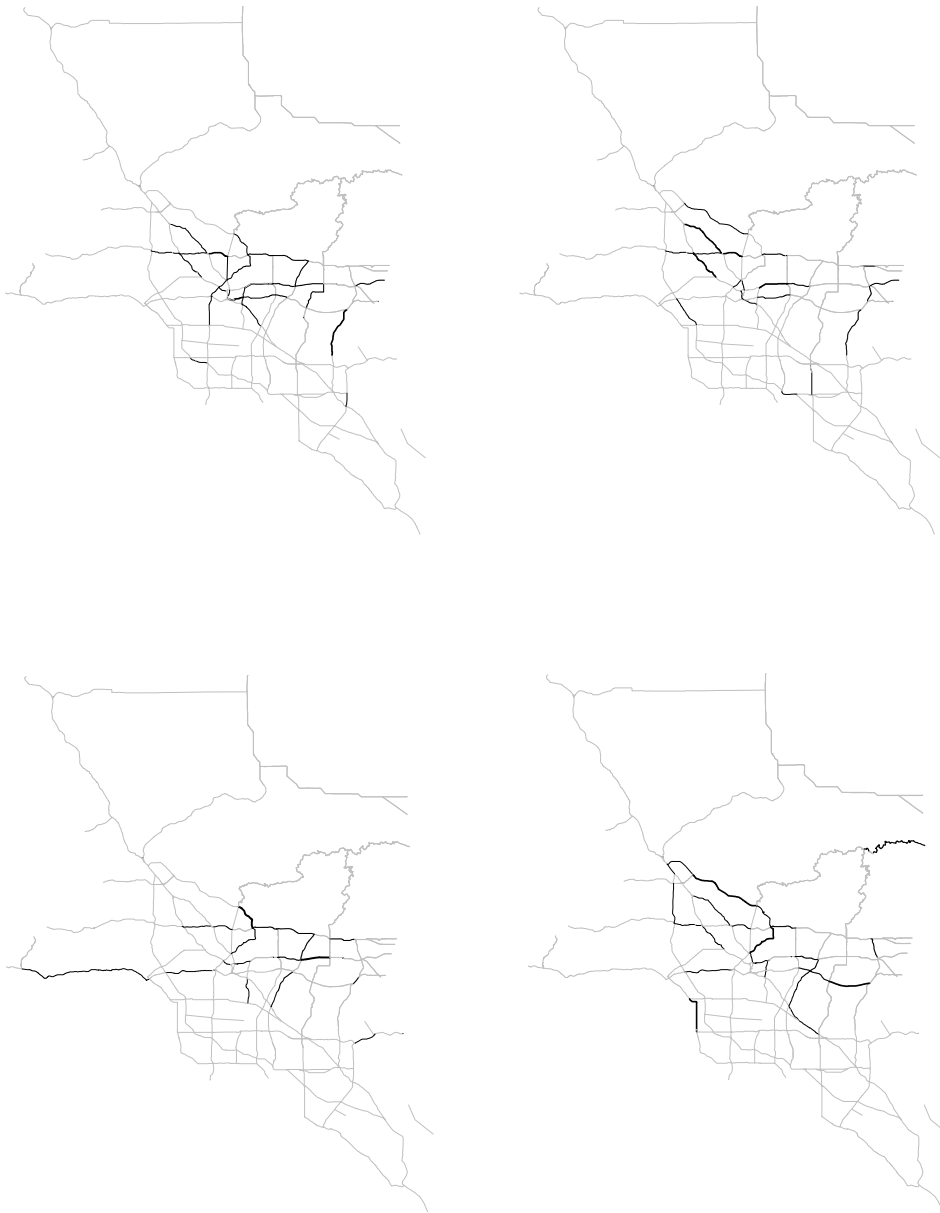
Figure 4: Simulated Bridge Failures Given Conditions Consistent with the Elysian Park Blind Thrust Fault Scenario: Darker Links Have More Failures
